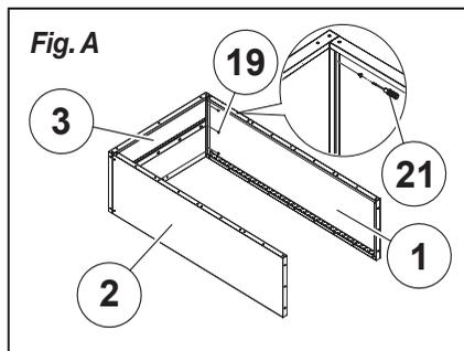
**Note:** Make sure the front of the cabinet frame is facing down. Once the cabinet frame is assembled, turn the cabinet frame to the upright position to attach the back panels.
