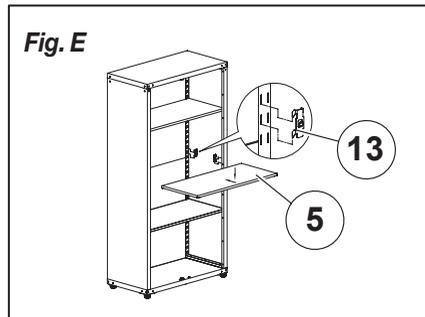
**6.** Choose the desired height for placing each middle shelf (Part 5) inside the cabinet. Then pull down the hooks (Part 13) into the hook slots provided, making sure the four hooks are placed at the same height. Place the shelves into the cabinet frame and press them down onto the hooks (Fig. E).
