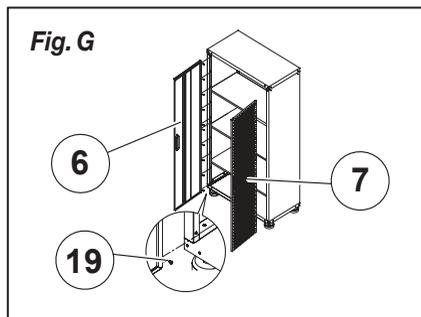
**9.** Place the bumpers (Part 14) on the corners of the bottom panel. Insert four M4 x 18 screws (Part 18) into each bumper and tighten them using the screwdriver (Part 21). Then place the corner protectors A (Part 16) on the front right and rear left and corner protectors B (Part 15) on the front left and rear right of the top panel (Part 3). Insert five M4 x 8 screws (Part 19) into each corner protector and tighten them using the screwdriver (Part 21) (Fig. H).
