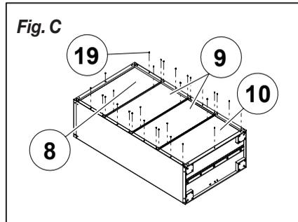
**Note:** Two screw holes for corner protectors are reserved across the top panel and the bottom panel.
