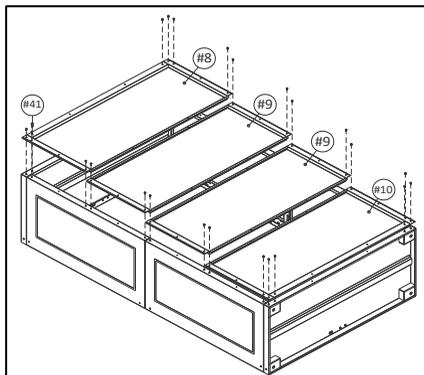
**2)** Attach both middle back panels (9) above bottom back panel (10) the same way. Place the groove of the middle back panel (9) onto the top edge of the bottom back panel (10).
