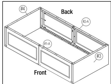
**Note:** Before tightening screws, make sure the bottom corners of left side-bottom panel and right side-bottom panels (1-A2, 2-A2) are completely flush with the back and front corners of bottom panel (4).
