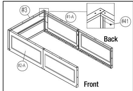
**Note:** Before tightening screws, make sure the bottom corners of left side upper panel (1-A1) and right side upper panels (2-A1) are completely flush with the back and front corners of top panel (3).
