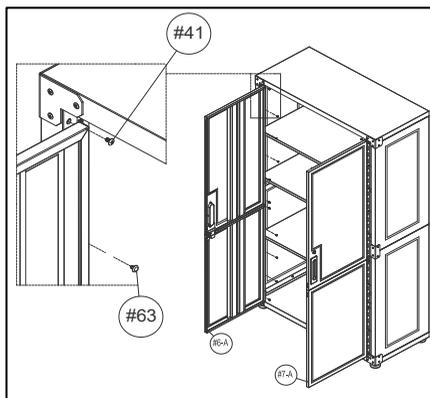
**Note:** The screw holes on the door hinge have tolerance, enabling the door to be adjusted and centred in the door frame. Place top, middle and bottom screws first. Don't tighten screws completely — this may save time by avoiding having to make slight adjustments for levelling door panels later.
