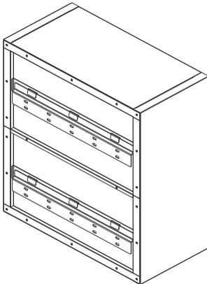
Back panel view of wall cabinet shows 6 flat hooks that allow the cabinet to hang on two wall-hanging brackets.
