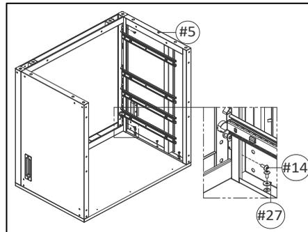
**5. Install the Upper Back Panel (2) and Bottom Back Panel (3).**
