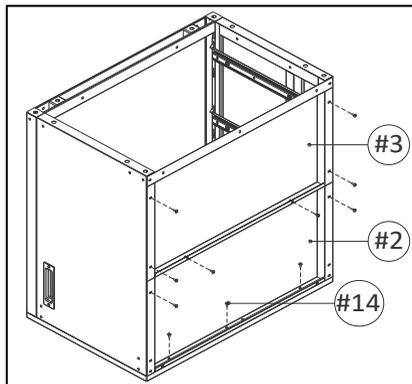
**2)** Attach bottom back panel (3) between the left panel (4) and right panel (5). make sure the top of the bottom back panel (3) is attached to the upper back panel (2) as the sticker indicates. Line up the screw holes and use screws A (14) to fasten the bottom back panel (3) to the upper back panel (2), left panel (4) and right panel (5).
