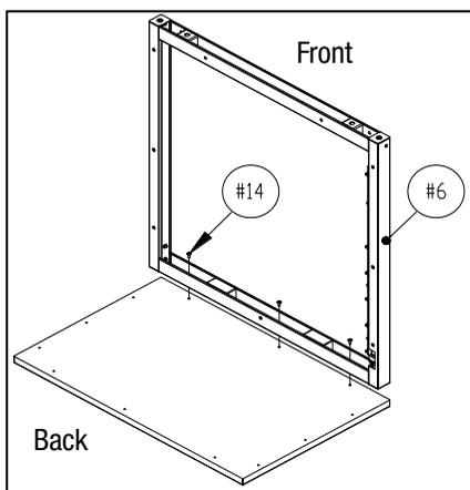
**Note:** Ensure the back and side of front frame (6) are flush with the solid hardwood top (1). When assembling, do not tighten any screws completely until all screws for that part have been partially screwed in.
