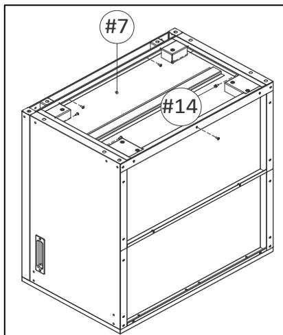
**Note:** Only the inner holes of the left side panel, right side panel, front frame and bottom back panel are use for attaching the bottom panel. The other four side holes at the corners are reserved for bumpers.
