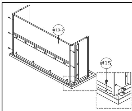
**Note:** Do not fully tighten any one screw until all screws are partially screwed in.
