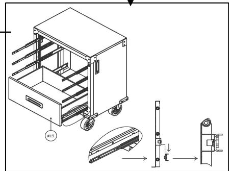
**Note :** Please remove the hook's rubber protectors before you assemble drawers onto slide.
