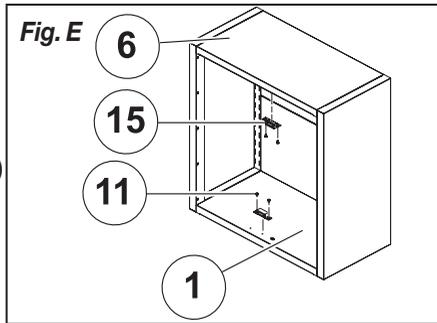
**Note:** The black plate of the magnet (15) should be facing the front.
