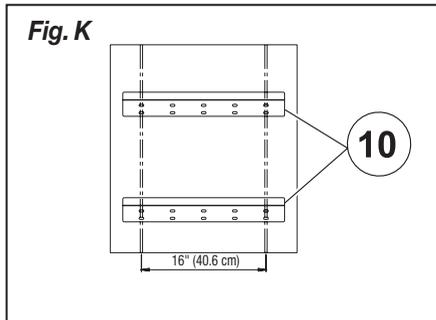
**3.** Insert the wall anchors (14) into the holes drilled into the wall. Then, attach the wall-hanging brackets (10) to the wall by using four M6 x 60 screws (13) for each wall-hanging bracket. Hang the cabinet on the wall-hanging brackets (see Fig. L).
