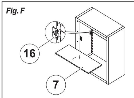
**Note:** When placing the hooks, make sure they are at the same height.
