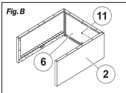
**3.** Attach the bottom panel (1) between the left panel (2) and the right panel (3). Line up the screw holes of all the panels. Insert three M4 x 8 screws (11) into the screw holes on each side of the bottom panel and tighten them using the screwdriver (17). Cabinet frame is assembled (see Fig. C).
