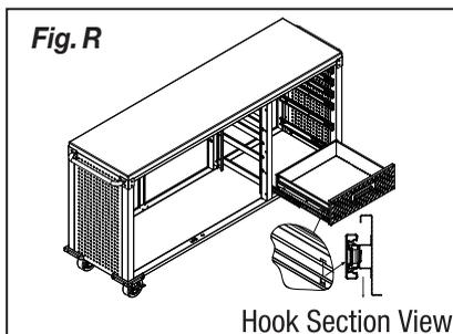
3. Secure the sliders to the drawer using four Screws (15) each and tightening with Screwdriver (21). Place the Drawer Mat (24) inside the drawer. Repeat for all six drawers (Fig. S).
